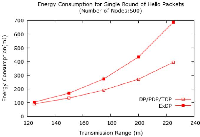
Fig. 11: Total energy consumption for a single round of hello packets of networks having 500 nodes (the transmission range is varied)
