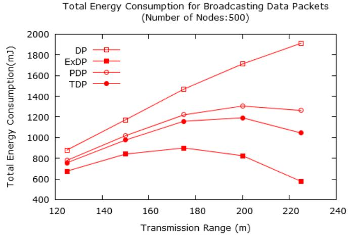
Fig. 14: Total energy consumption for broadcasting a data packet to the entire network of having 500 nodes (the transmission range is varied)
