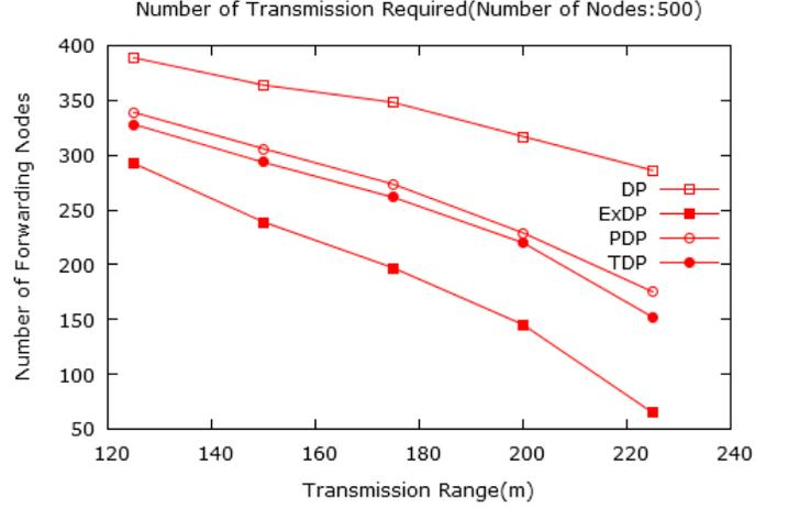
Fig. 5: Number of forwarding nodes of networks having 500 nodes by varying transmission range
