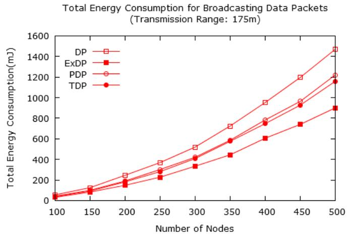
Fig. 15: Total energy consumption for broadcasting a data packet to the entire network (the number of nodes is varied)
