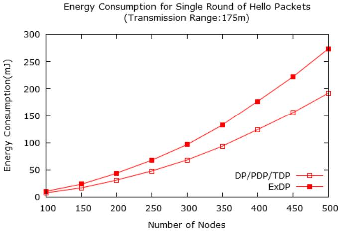
Fig. 12: Total energy consumption for a single round of hello packets (the number of nodes is varied)
