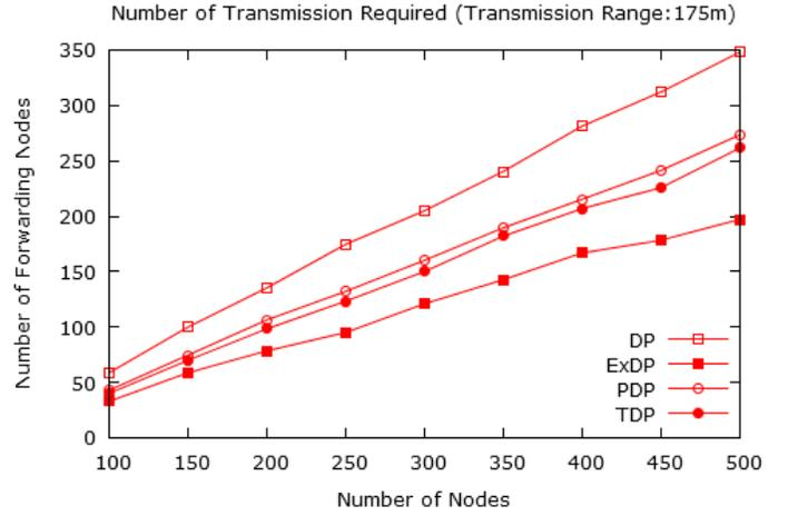
Fig. 6: Number of required transmissions by varying number of nodes in a transmission range of 175m
