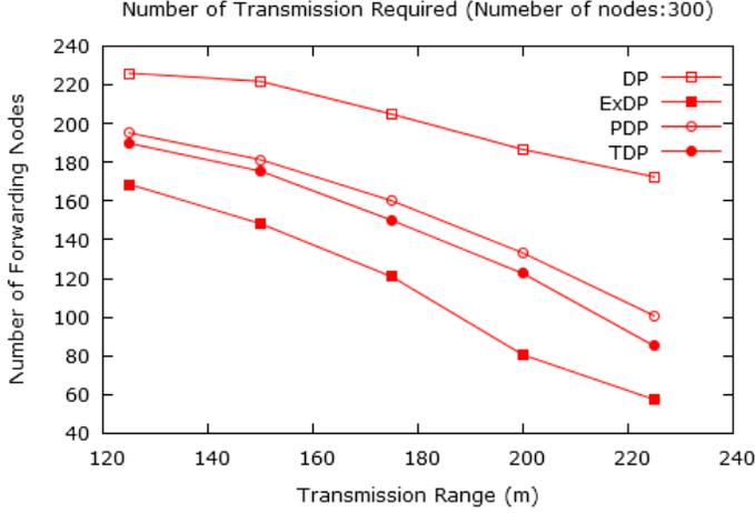
Fig. 4: Number of forwarding nodes of networks having 300 nodes by varying transmission range
