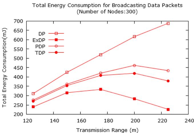
Fig. 13: Total energy consumption for broadcasting a data packet to the entire network of having 300 nodes ( the transmission range is varied)
